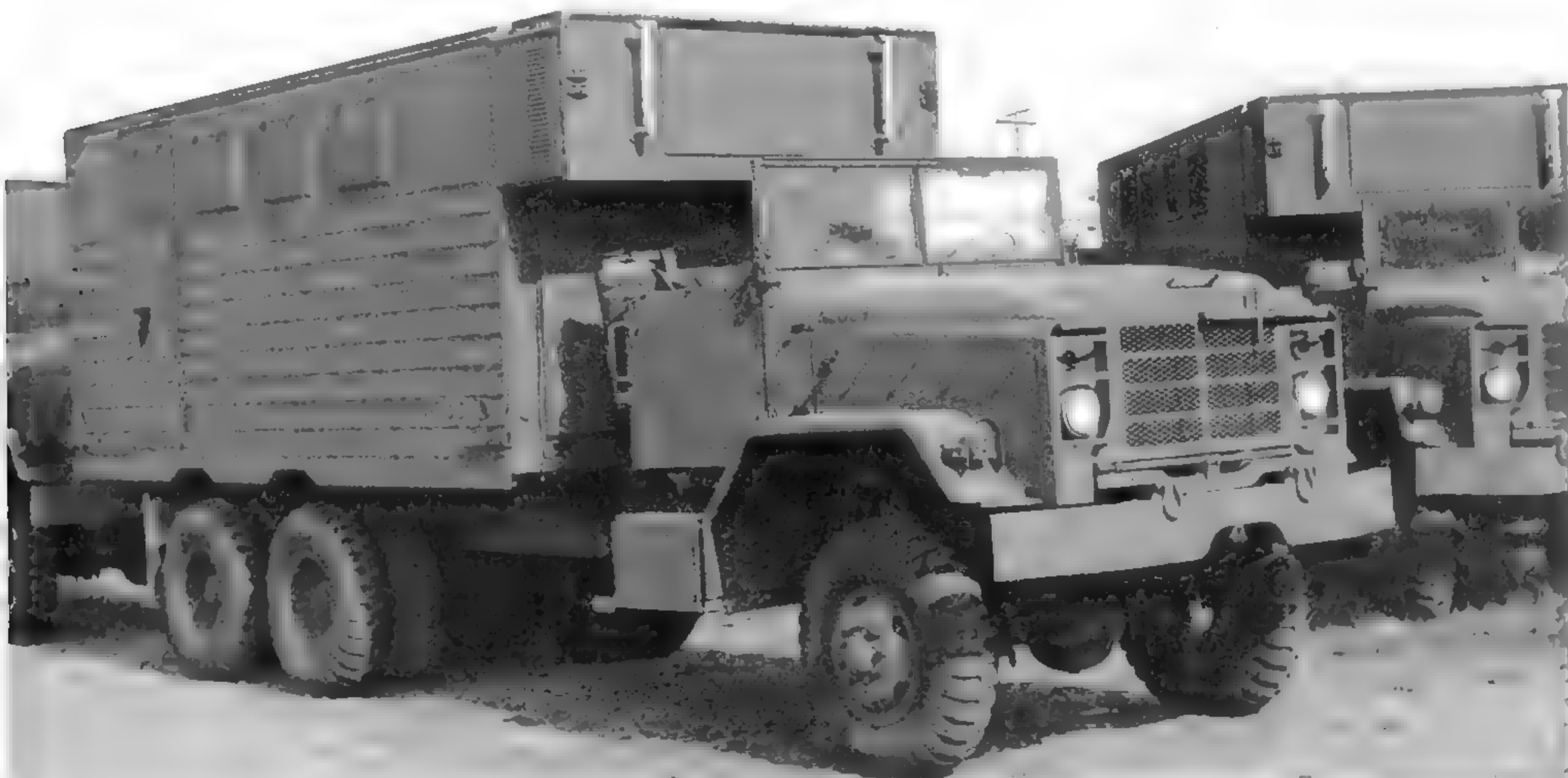
The exhaust stack used on these M934 expansible van trucks was considerably shorter than that of the rest of the series. This avoided interference with the heater and air-conditioner assembly extending over the cab. (Photo courtesy of the Patton Museum)
